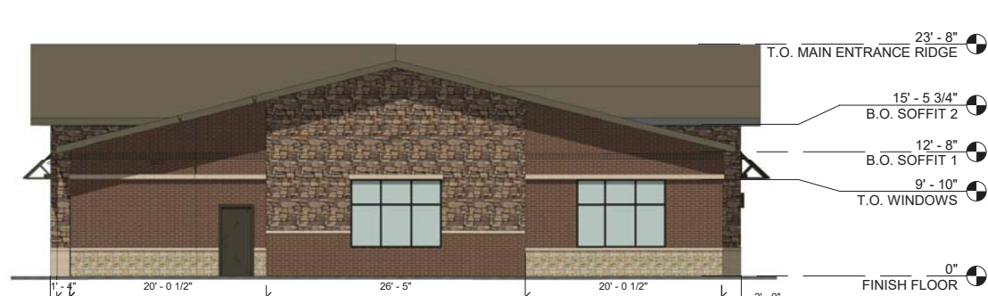
2 REAR-WEST ELEVATION FP 1/8" = 1'-0"
